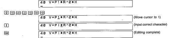
Again, the key must be pressed to store the corrected line into memory after changes are made.
